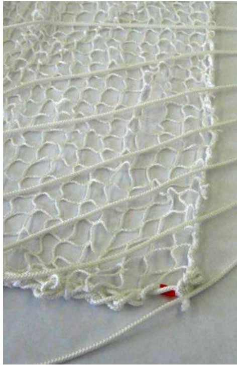
Figure 15 Strand Overlap Onto Netting
