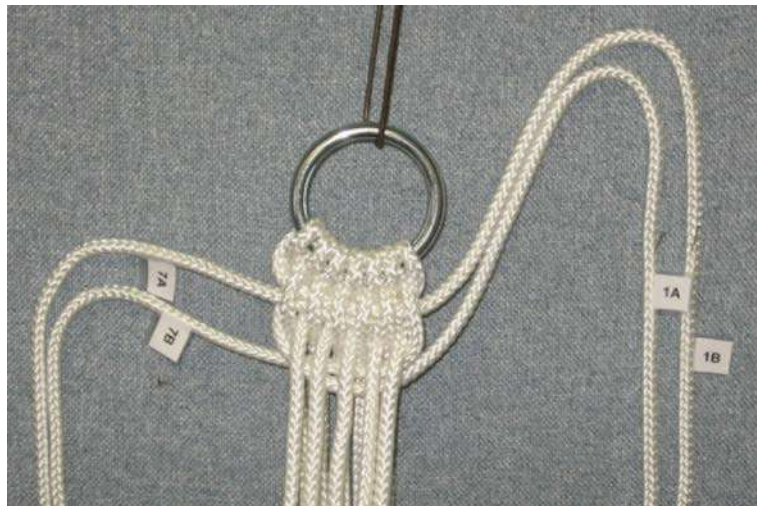
Figure 5 Passing the Strands Steps 6 through 9
